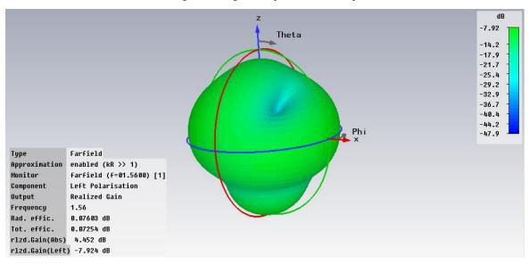
Figure 8. L-polarized antenna pattern
