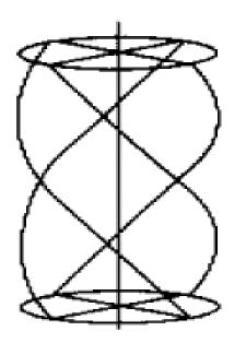
Figure 1. Resonant four-arm spiral antenna
