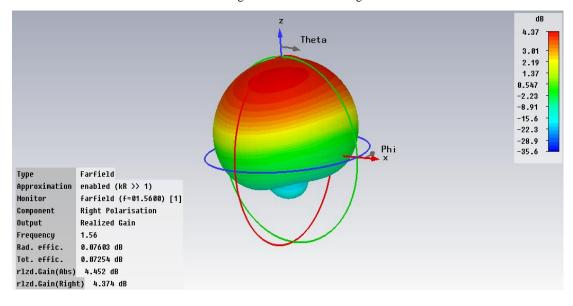
Figure 7. Right-hand polarized antenna pattern
